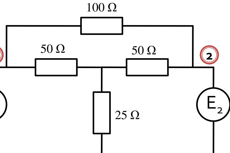
$$Y_{11} = \left. \frac{I_1}{V_1} \right|_{V_2=0}$$
