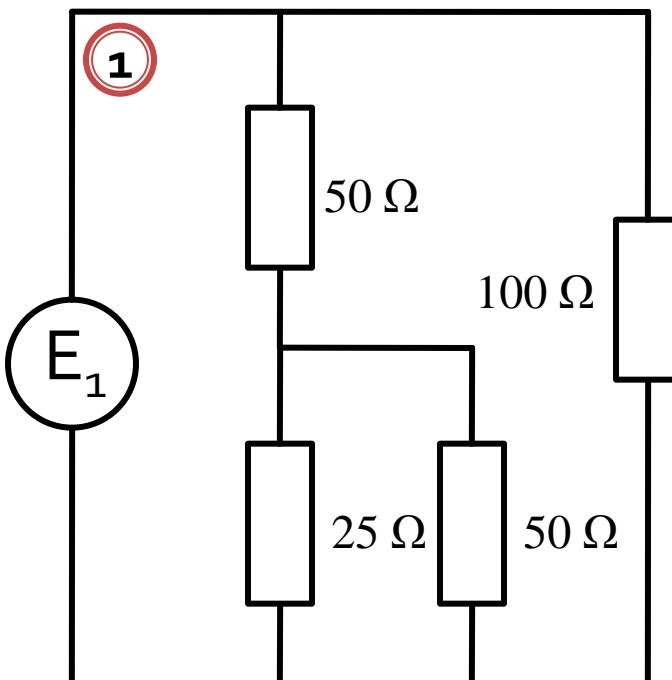
$$\begin{aligned} R_{ech} &= 100\Omega \parallel (50\Omega + 25\Omega \parallel 50\Omega) = \\ &= 100\Omega \parallel (50\Omega + 16.67\Omega) = 100\Omega \parallel 66.67\Omega = 40\Omega \end{aligned}$$
