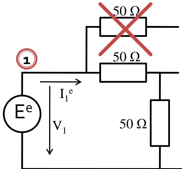
$$R_{ech}^e = 50\Omega + 50\Omega = 100\Omega$$
