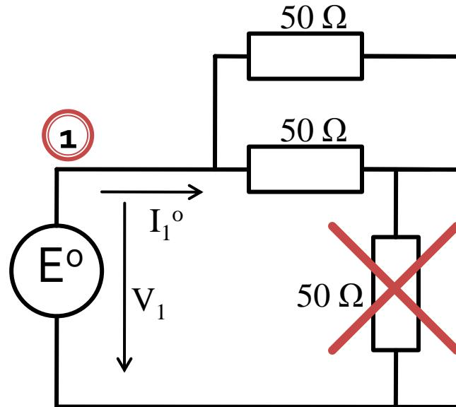
$$R_{ech}^o = 50\Omega || 50\Omega = 25\Omega$$
