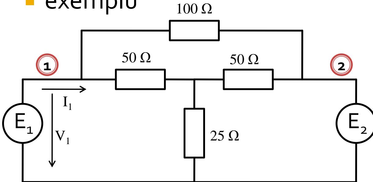
$$Y_{11} = \frac{I_1}{V_1} \Big|_{V_2=0}$$
