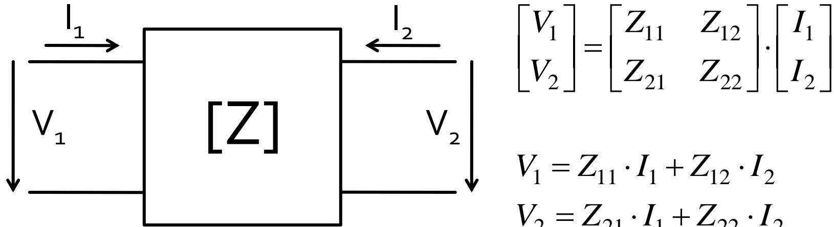
$$V_1 = Z_{11} \cdot I_1 \Big|_{I_2=0} \quad Z_{11} = \frac{V_1}{I_1} \Big|_{I_2=0}$$
