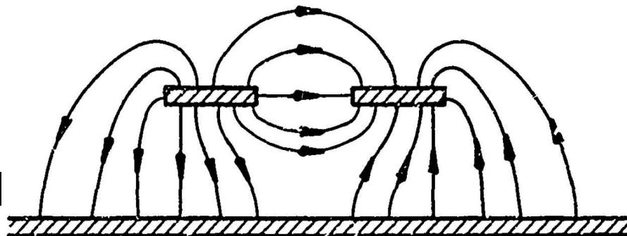
c) ODD MODE ELECTRIC FIELD PATTERN (SCHEMATIC)
