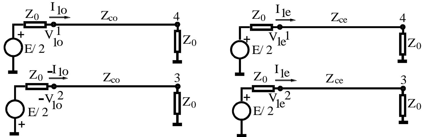
$$\left\{ \begin{array}{l} Z_{ce}Z_{co} = Z_0^2 \\ \theta_e = \theta_o \end{array} \right.$$
